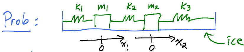
$$\left\{ \begin{array}{l} m_1 \ddot{x}_1 = -k_1 x_1 + k_2 (x_2 - x_1) \\ m_2 \ddot{x}_2 = -k_2 x_2 - k_3 (x_2 - x_1) \end{array} \right. \quad \begin{array}{l} \text{Take all} \\ \text{const} \\ = 1 \end{array}$$
